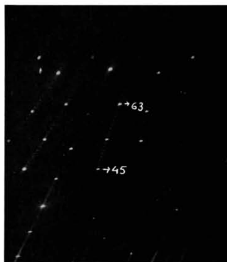
Fig. 8. Zero-layer a -axis Weissenberg photograph of polytype 18H 9 . Cu K\alpha radiation; camera diameter 5.73 cm. The lowest festoon shows the 10.l row of spots. The l values of two strong spots are noted on the photograph.
