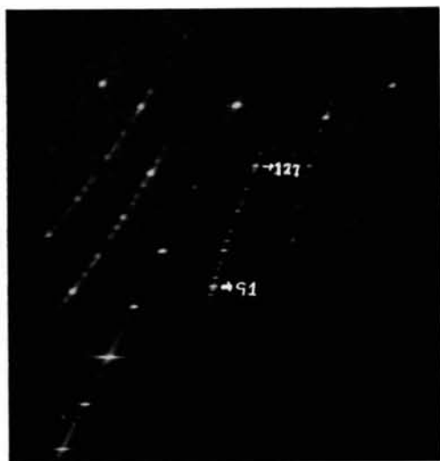
Fig. 6. Zero-layer a -axis Weissenberg photograph of polytype 36R. Cu K\alpha radiation; camera diameter 5.73 cm. The festoon corresponding to the 10.l row of spots is recorded on the right side of the straight row of 00.l spots; the l values of two strong spots are noted on the photograph.
