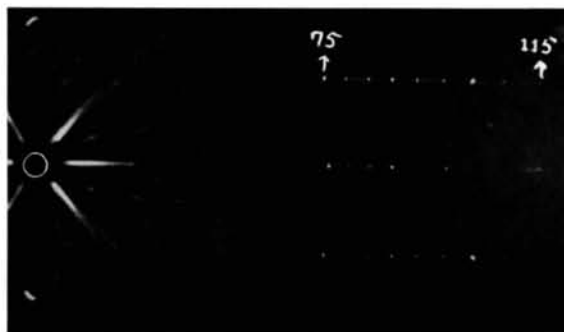
Fig. 9. A 15^\circ a -axis oscillation photograph of polytype 30H dx . Cu K\alpha radiation; camera radius 3 cm. The l values of two strong spots along the 01.l row are indicated on the photograph.
